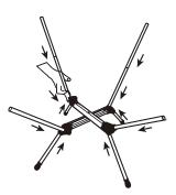
2. Assemble the frame by opening the X-frame and inserting each pole into each open slot of the hub.
